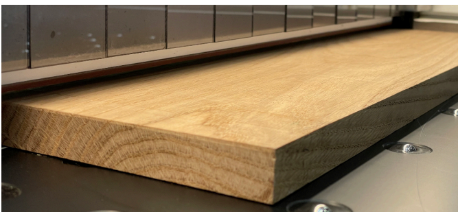
Electronical positioned clamping device over the total part width.
