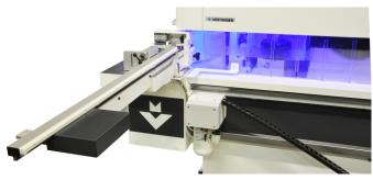
The automatic length fence allows the operator to size workpieces to length, and the large swiveling backstop allows for the sizing of two pieces at the same time.
