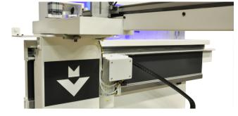
The automatic table will adapt the speed based on the selected program and will change the speed for sawing, coping and traveling.
