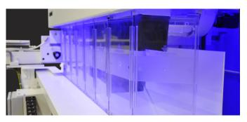
The transparent safety-screen covers the entire machining area. Loading and unloading remain efficient and operator-friendly.
