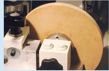
Round backing wood with 6 manual adjustable positions.
