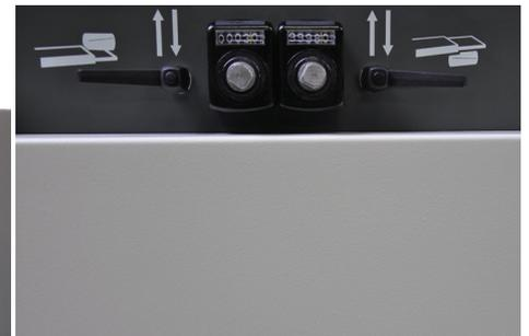
The spindles are horizontally and vertically adjustable with 0,1 mm accuracy.
