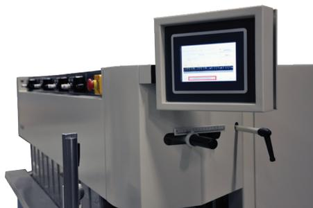
7" touch panel for the operation of the machine and starting of all motors
