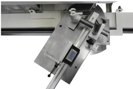
The table can be swivelled 60° in two directions. The working area of the table does not change.
